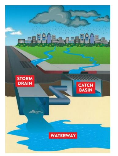
The water then flows into storm drains and catch basins.
